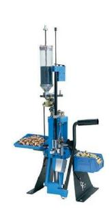
The most versatile reloader available, capable of loading over 160 calibers. An automatic casefeeder is available for handgun calibers. Manual indexing and an optional magnum powder bar allow you to load magnum rifle calibers.
